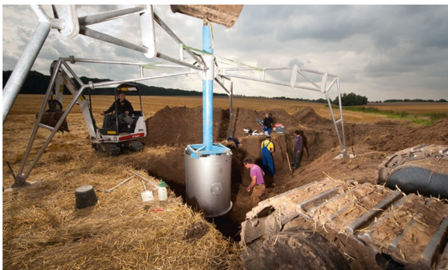
Assembling lysimeters at the TERENO-site of Sauerbach in the Harz Mountains. With the use of lysimeters scientists are investigating the impact of climate change on the soil.
